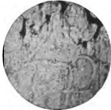
Fig. 20. Steel quenched at 100 De- grees C. above Correct Hardening Temperature
